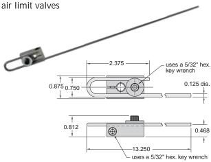
Arm: Steel 1/8" rod 13 inches long retained by screw clamp; the rod may be shortened and/or bent to desired shape
